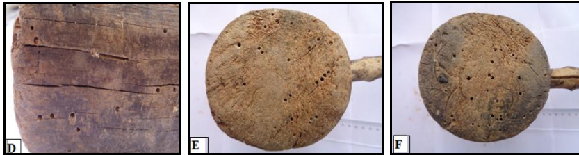
Fig.32. Damage characteristics of the old wooden mallet by Anobium punctatum .
