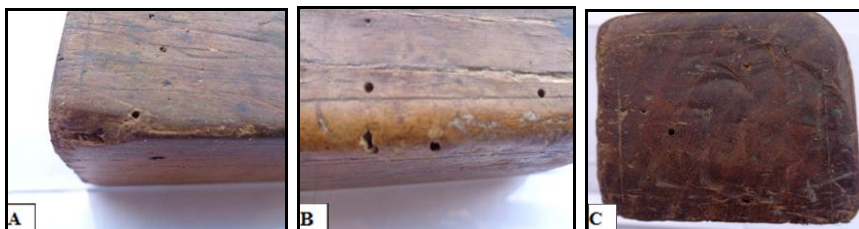
Fig.36. Damage characteristics of the old wooden plane by Anobium punctatum
